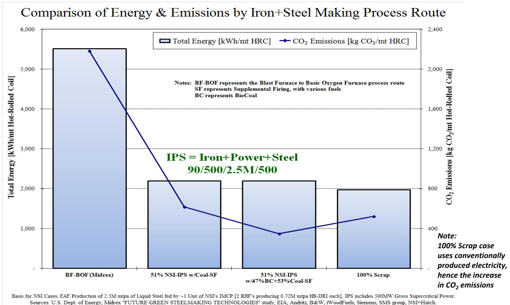
*The Use of Advanced and Renewable Energy from the IMCP Significantly Improves the Environmental Impact of the Steel Making Operation*
